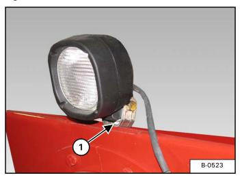
Using one bolt (Item 1) [Figure 223] and lock nut (included with light), install the work light on top of the intake auger.
